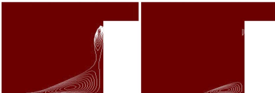
(c) Close-up view of normal velocity recirculation ( w < 0 ) contours at re-entrant and salient corners, h = 1/128 .
